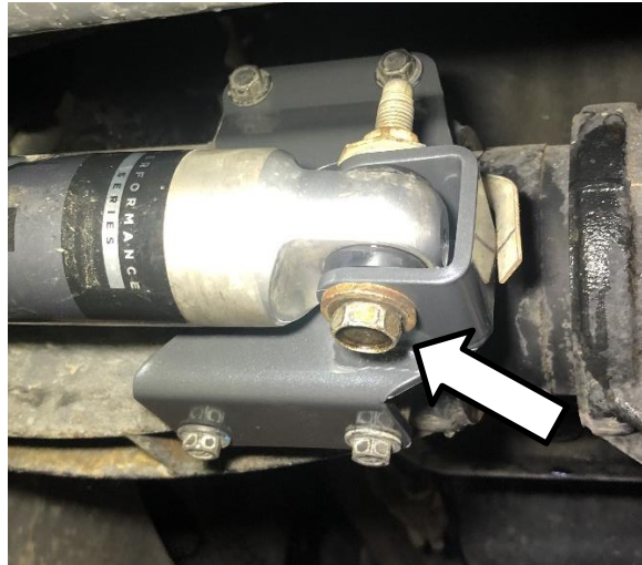
Figure 4. Reinstalled Stabilizer on Synergy MFG Bracket
