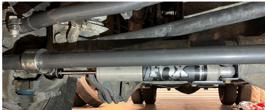
Figure 8. Installed 8703-02, Steering Stabilizer and Tie Rod Clamp
