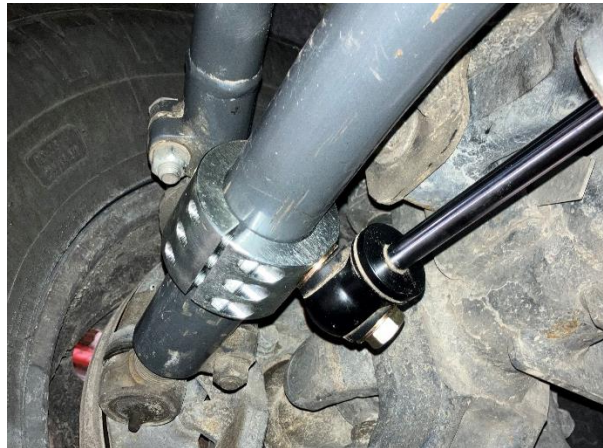
Figure 7. Installed Tie Rod Clamp and Steering Stabilizer
