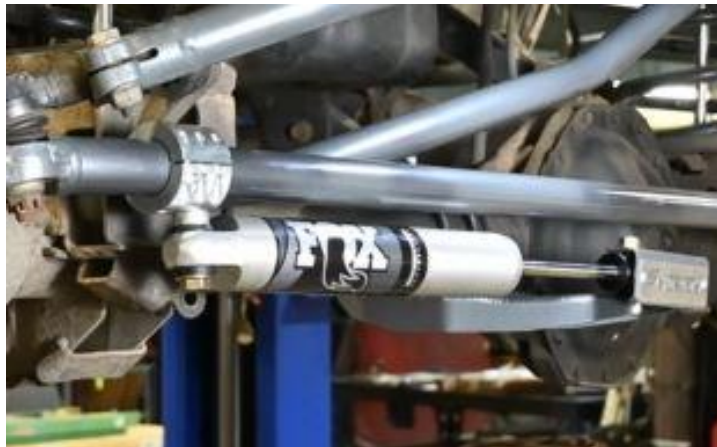
Figure 6. Correctly Installed Stabilizer
