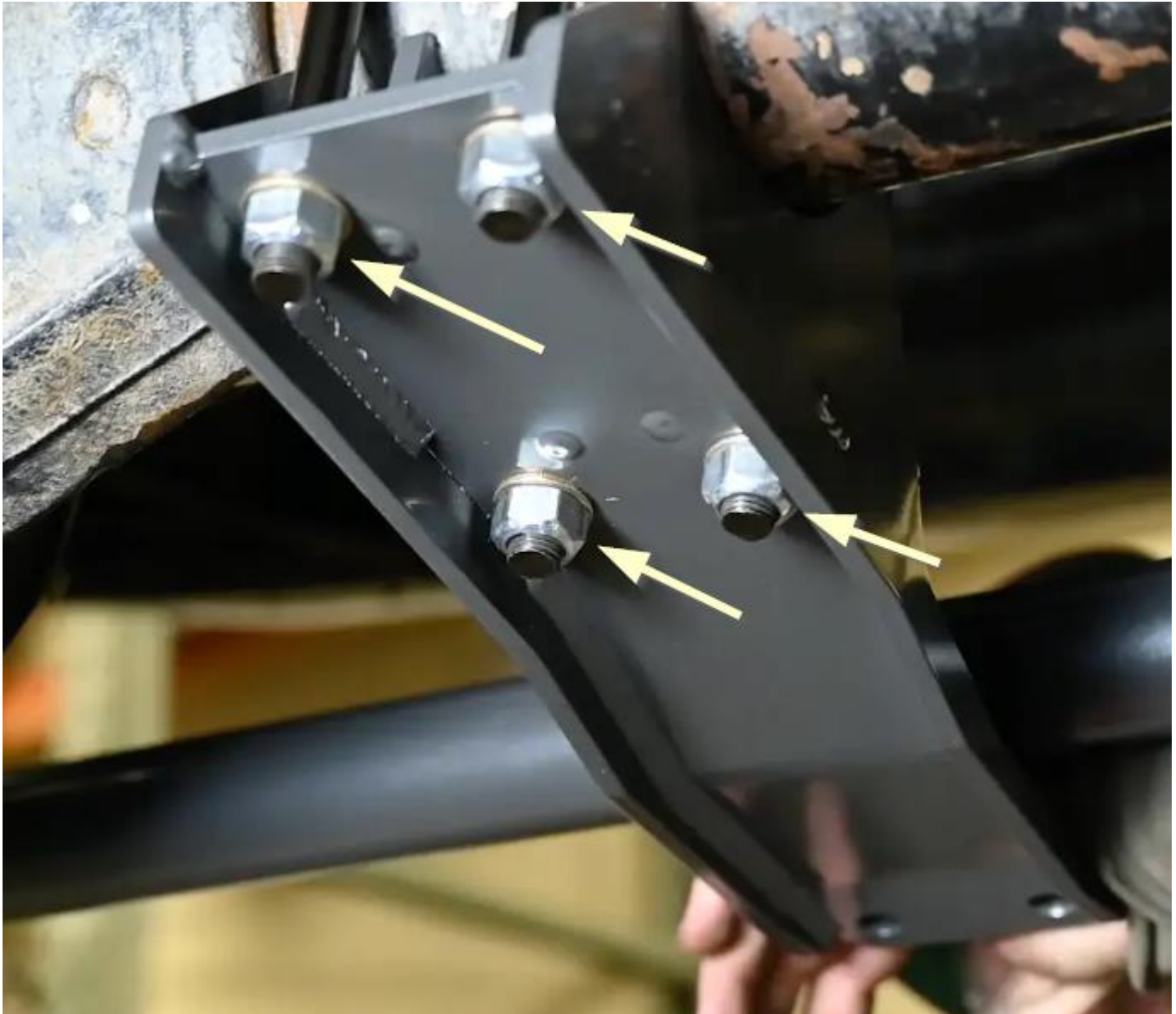
Figure 1. Bolts to Hold the Dual Stabilizer Bracket
