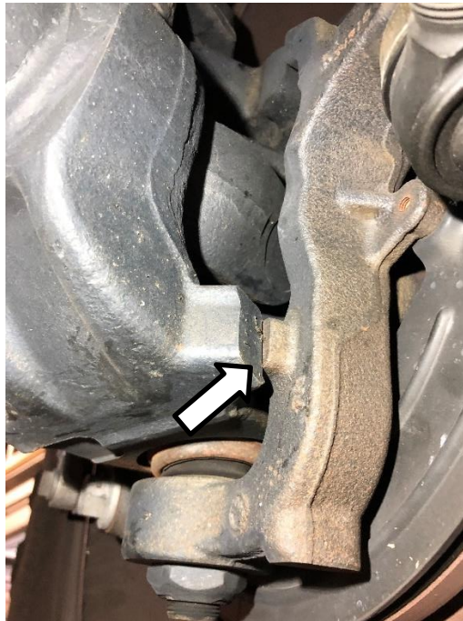
Figure 5. Driver Side Knuckle Fully Turned to the Passenger Side, Contacting the Steering Stop
