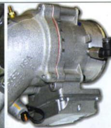
02. The two nozzles are located at the end of the air horn. The primary nozzle sprays continuously while the secondary power nozzle opens on full throttle.
