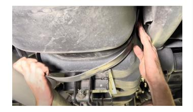
Drop the tank 2-3 inches and if you have any remaining lines on top of the sending unit, make sure you disconnect those.
