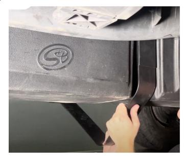
Reinstall the middle strap in the same way you installed the rear strap.
