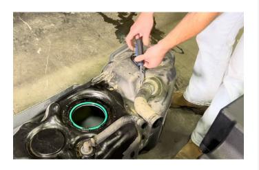
Once the filler neck is off the stock tank, press the check valve in (make sure the "FLOW" arrow is pointing towards the tank)
