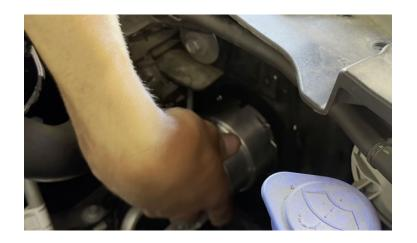
Now, assemble the (2) T-bolt clamps onto the intercooler pipe with the 90 degree bend. Then, install it onto the turbo as shown.
