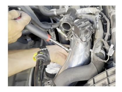
Before tightening down any of the t-bolt clamps, make sure that they are all orientated in a way that will make them easy to access with a socket to tighten them down.
