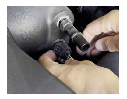
Cut off the zip tie holding the hose to the rear of the air box/intake tube.
