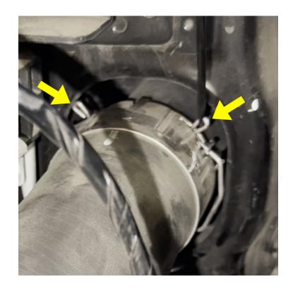
Using an **8mm** socket or **5/16th** nut driver, remove the (3) bolts holding the Blowoff Valve to the stock pipe.
