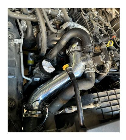
Next, go ahead and re-install your air intake. First start by mounting your S&B air box. Then go ahead and tighten down the (2) **10mm** bolts at the bottom of the box.
