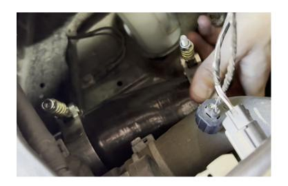
Now, go ahead and install the large S&B aluminum pipe and ensure that the mounting bracket lines up while connecting all (3) intercooler pipe segments together.
