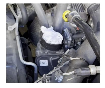
Using a **13mm** socket, loosen and remove the bolt holding the intercooler pipe bracket.
