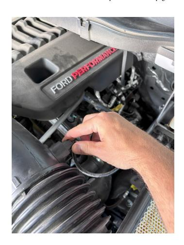
Lift up and remove the stock air tube.
