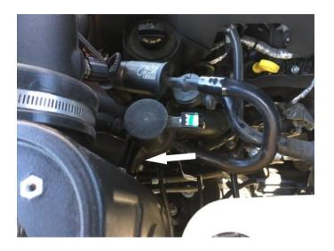
Use the two provided Plastic Rivet (5) to secure the Front Inlet (3) onto the radiator cover. Firmly push down on the center pin of the plastic rivet until it locks into the closed position.
