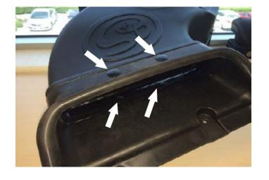
Install the Grommet (9) into the Intake Tube (14).
