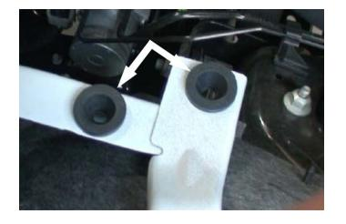
Re-install the retaining bolt removed in Step 9 and tighten the bolt to secure the air box (16). Install the retaining bolt from inside the air box.
