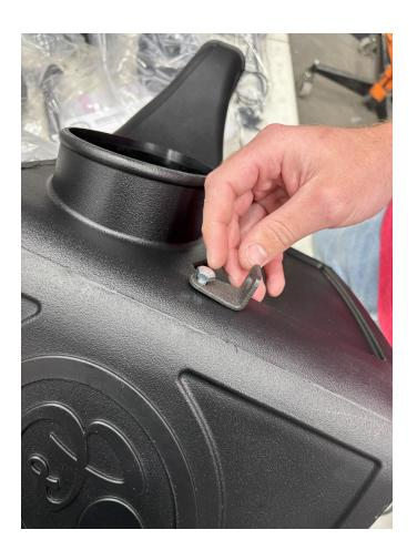
Install the Cuff (1) and #104 Hose Clamp (7) onto the side of the air box (16). Make sure that the rubber pull tab on the tube seal is on the bottom. Tighten the hose clamp.
