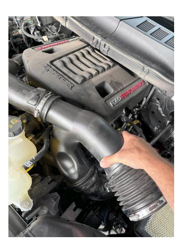
Remove the retaining bolt on the stock air box using a **13mm** socket.
