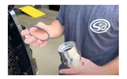
Install the S&B boot onto the intercooler with no hose clamp springs.
