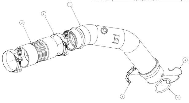
Start by loosening the hose clamp on the intercooler side.
