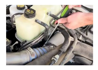
Remove the clip on the top of the intercooler. To remove the clip, pry up on the clip and slide it to the top of the retainer. Repeat for the bottom part of the clip.
