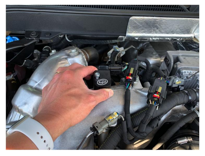
Install the MAP Spacer into the Intake Manifold as shown. Make sure the O-Ring (B) does not accidentally fall out of the groove. When the O-Ring is fully seated in the groove, it will not fall out. Use the M6 SHCS (C) to secure the MAP Spacer to the Manifold. Torque the M6 SHCS to 60 in-lbs. Torque the M6 Hex Flange Screw (from Step 4) to 60 in-lbs.
