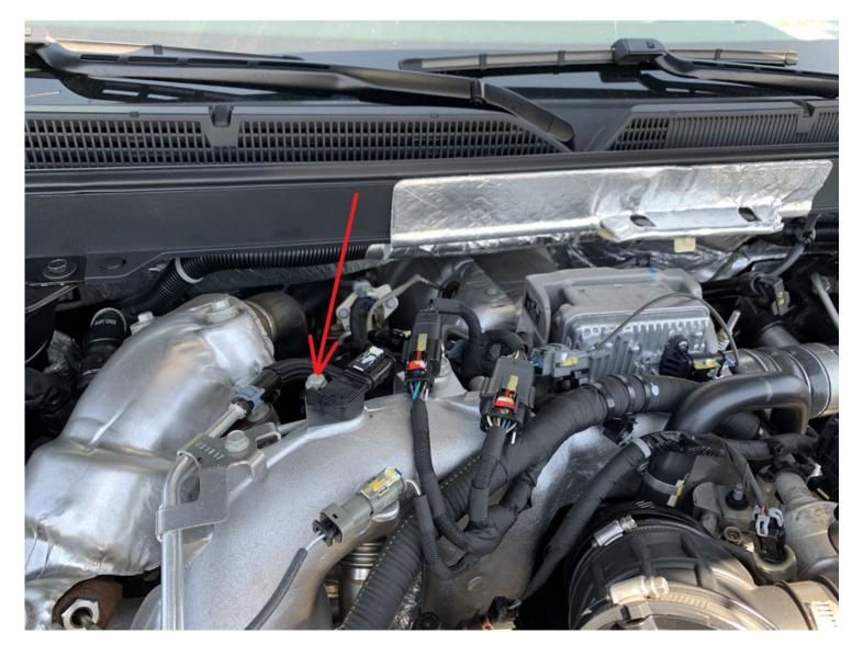
Make sure the engine is off, cooled down, and the vehicle is safely parked with the parking brake set. Locate the MAP Sensor and the M6 Hex Head Flange Screw holding the MAP Sensor in place.
