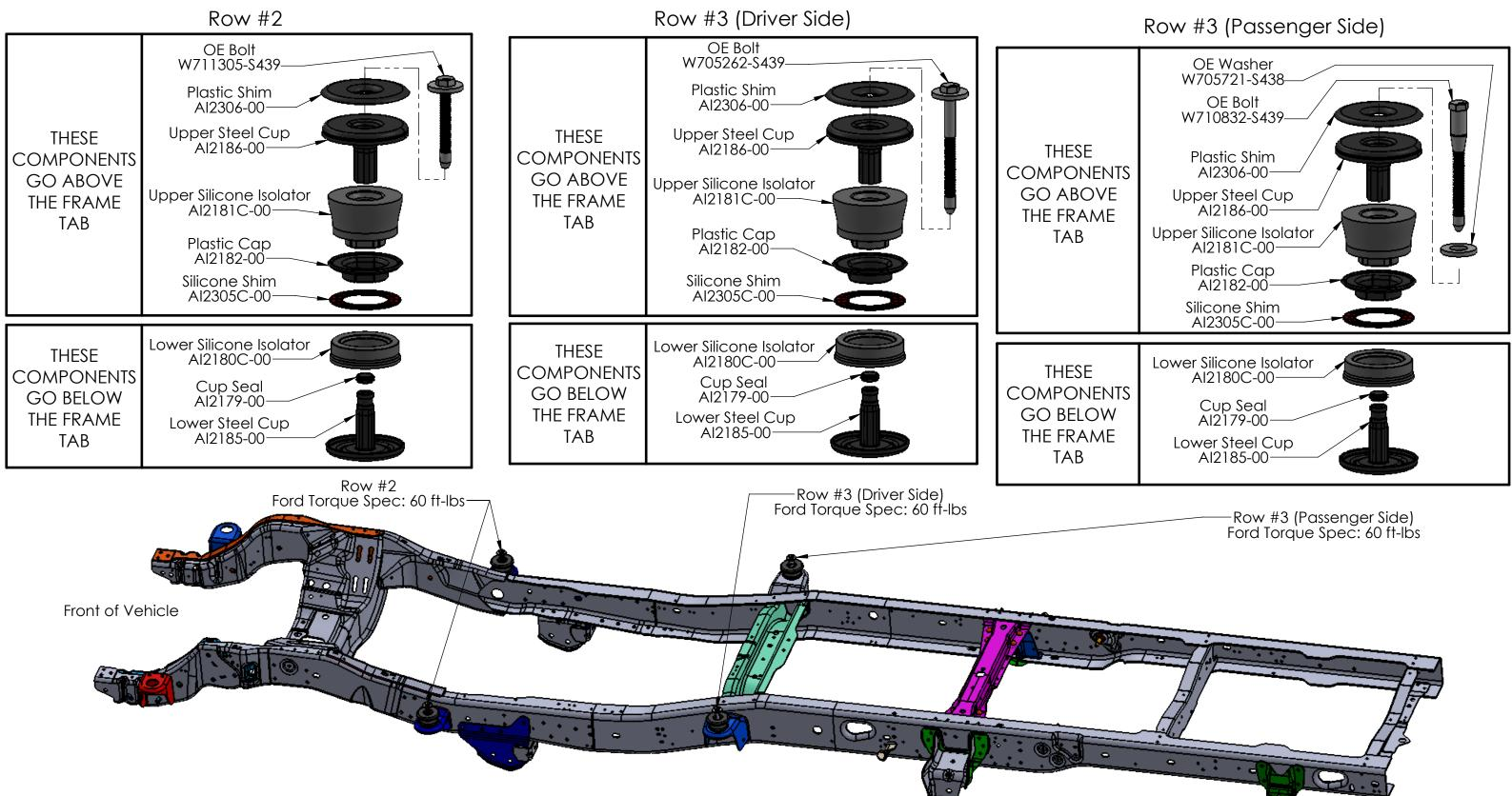
WARNING: Qualified professional installation of this product in accordance with the Ford service documentation and using a vehicle lift is reauired.
