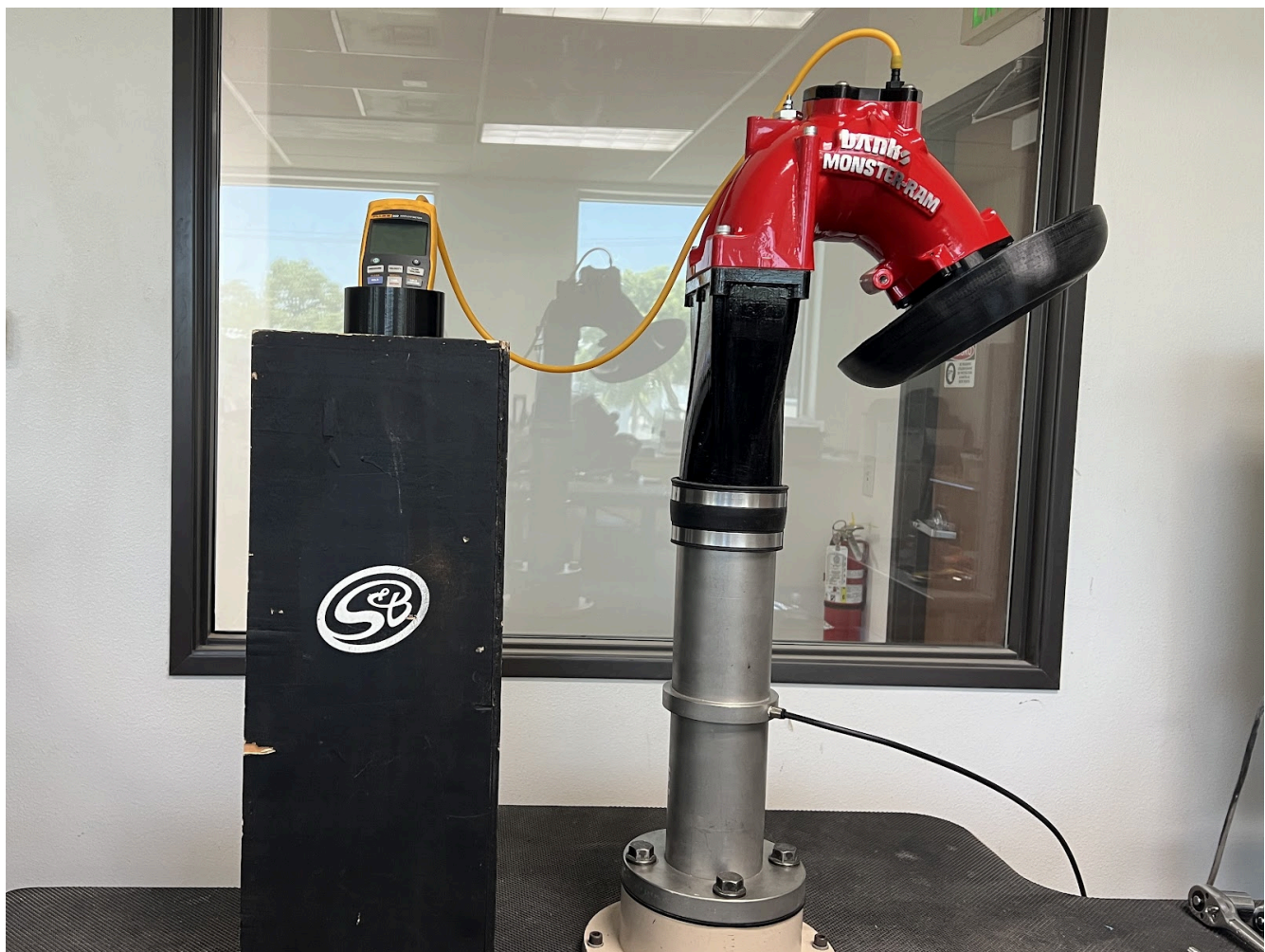
Banks Elbow Airflow Test w/Heater (No TMAP Sensor)
