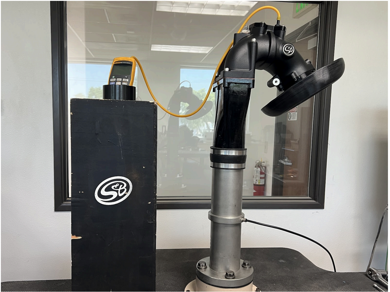
S&B Intake Elbow Airflow Test w/Heater (No TMAP Sensor)
