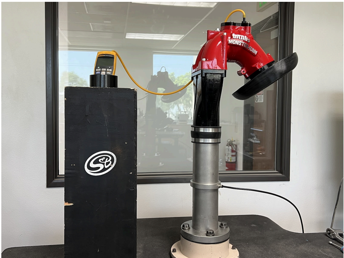
Banks Elbow Airflow Test (No Heater & TMAP Sensor)
