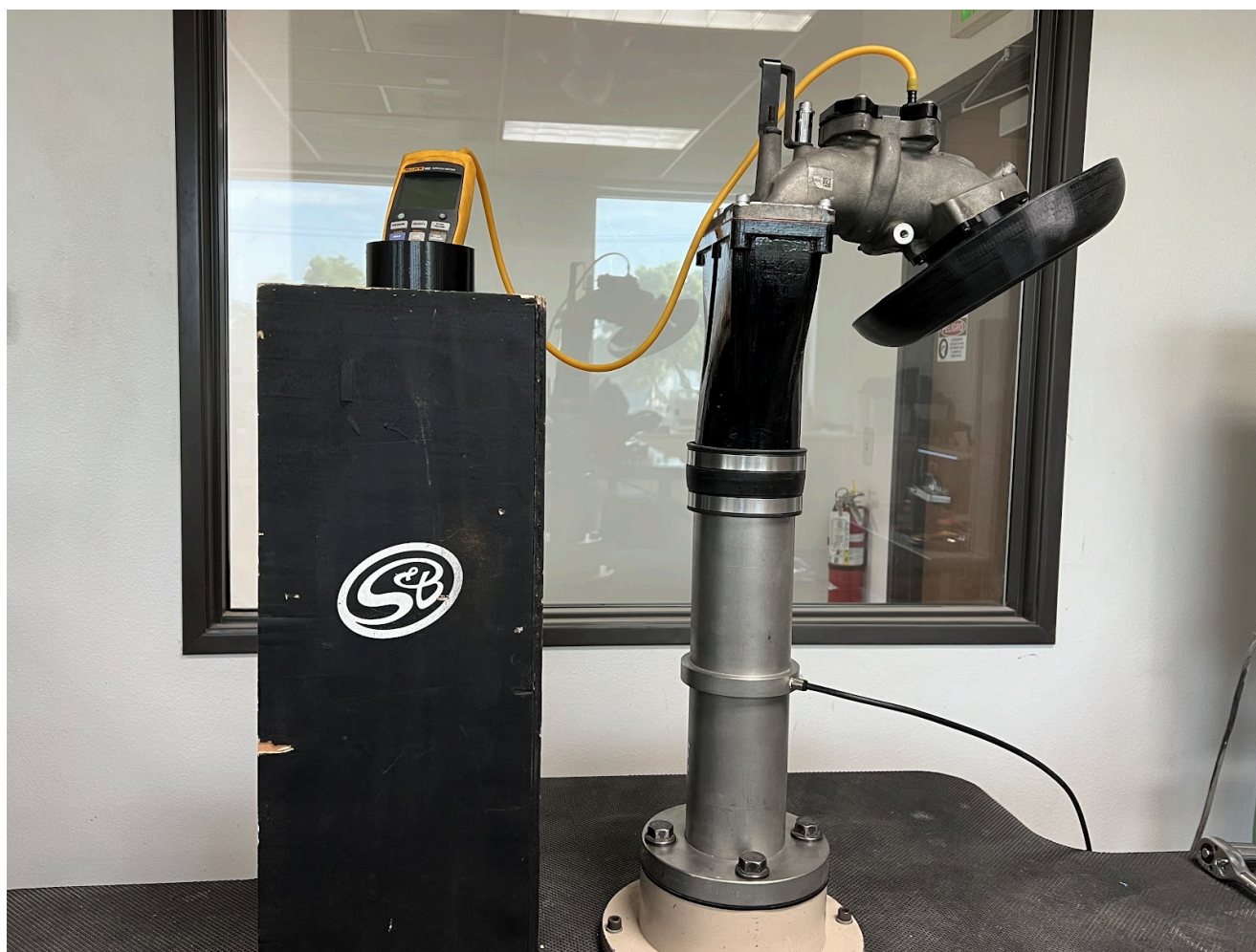
OE Cummins 6.7L Intake Elbow Airflow Test (No Heater & TMAP Sensor)
