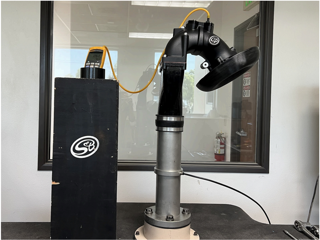
S&B Intake Elbow Airflow Test (No Heater & TMAP Sensor)
