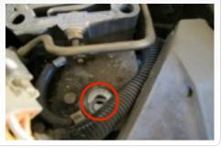
18. Slide the OE t-bolt clamp up onto the Silicone Adapter (S) and torque the clamp to 90 ln. lbs.
