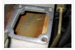
This kit has 2 Long Stud (J) and 2 Short Stud (H), to determine the correct stud length for your truck, thread each a long and short stud (short threaded end first) into the manifold bolt holes farthest from the valve cover. Measure the height of the stud from the heater grid block upward. Use the studs that are approximately 1.125". (See pg. 5 for details)
