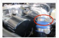
3. Remove the bolt that secures the dip stick tube to the elbow.
