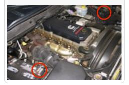
Loosen the upper hose clamp at the OE elbow and disconnect the hump hose from the elbow. Note: Care should be taken not to
