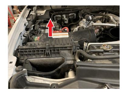
Remove the indicated grommet from the vehicle.
