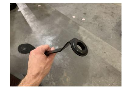
Install the tube support bracket (D) into the vehicle using the custom washer (K) and the screw removed in step 11. Slide the end of the bracket under the area of the vehicle where the grommet was removed from in step 10. Place the custom washer over the hole so that the step on the washer is seated inside the hole. Use the previously removed screw to finish the installation. Do not torque the screw down so that the bracket retains some play without falling out of position.
