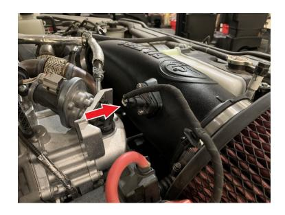
Visually inspect the installation of the intake kit. Make sure the tube is fully seated within the support bracket and that the tube did not push out the grommet during installation.
