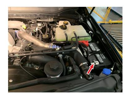
Disengage the white locking clip, press down on the tab, then pull out to disconnect the MAF sensor harness from the MAF sensor.
