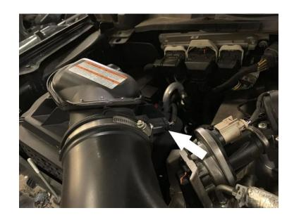
Disconnect the hoses attached to the stock intake tube.
