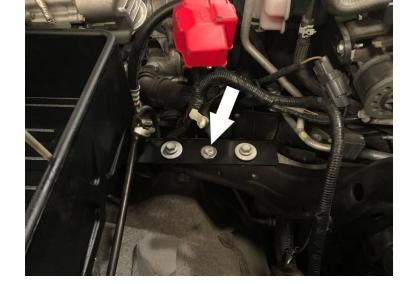
Reattach the grounding bolt removed in Step 19 as shown. Re-use the factory grounding bolt to attach the primary ground to it's original threaded hole on the fender and torque to factory specifications, 106 lb-in (12Nm). Note: The primary ground should be at an angle with the prong facing away from the fender as shown.
