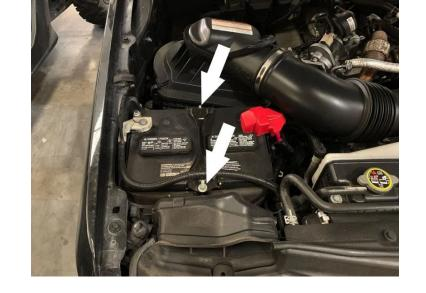
Remove the battery and battery blanket from the vehicle. The battery is heavy so be extra careful when taking it out. The battery is also filled with battery acid so remember to keep it level to prevent the acid from spilling out the top.
