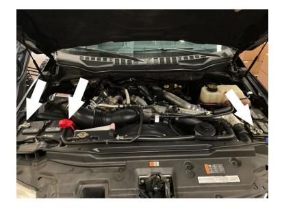
Remove the two nuts on the battery hold down bracket, then remove the negative battery cable mounting tab and hold down bracket from the battery. Set the hardware aside they will be reused in Step 27.
