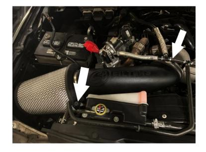
Attach the provided MAF harness extension (Q) to the existing MAF sensor connector by inserting the male end and engaging the red locking clip.
