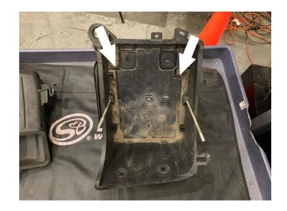
Pop out the hold down U-bolt from the underside of the battery tray.
