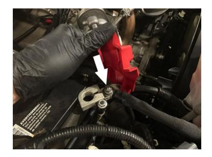
Disconnect the connection between the two wire harnesses shown. Cut the zip tie securing the indicated plug to the negative battery terminal cable.
