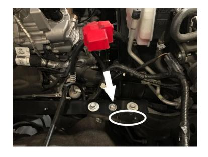
Remove the stock hold down U-bolt from the stock battery tray by first removing the two screws securing the stock battery tray to the stock intake inlet.
