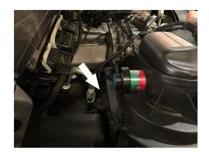
Lift up the stock intake box slightly to unseat the prongs from the stock grommets, then remove the stock intake box from the vehicle.
