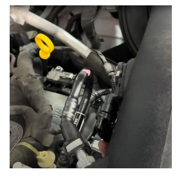
Press the previously removed large harness into the S&B airbox.
