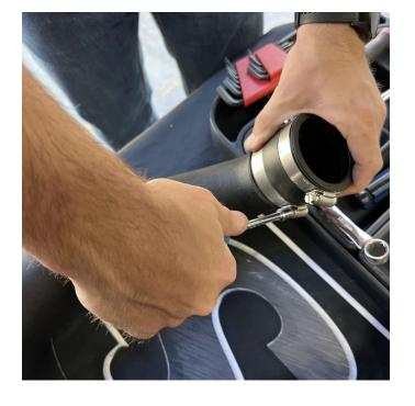
Add the supplied grommets and front scoop to the airbox.
