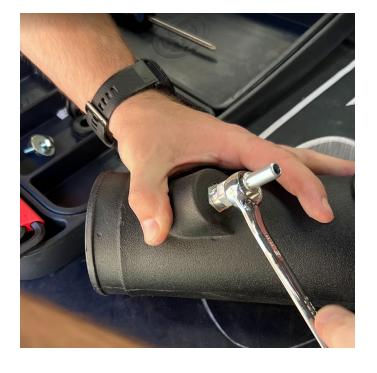
Then, start transferring the stock MAF sensor by unfastening it with a Torx from the OE airbox.
