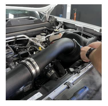
Connect the PCV fitting to the S&B tube, making sure it locks.
