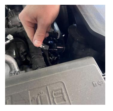
Disconnect the fitting on the purge valve by pressing on the tab and pulling it off.
