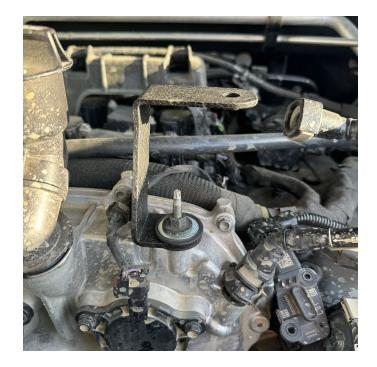
Install the other bracket on the passenger side engine mounting point, also fastening to the S&B tube. Fully tighten both brackets making sure the top tabs are pointing in an opposite direction towards the respective fenders of the vehicle. You can verify their orientation by making sure the holes line up with the cover. Make sure the harnesses are not being squeezed underneath the bracket.
