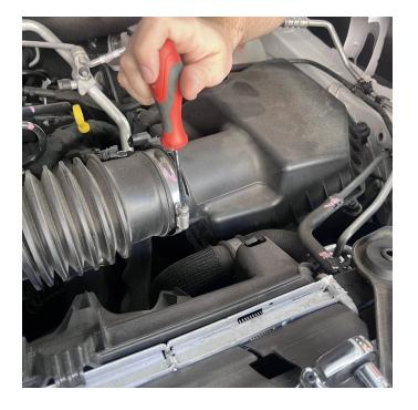
Disconnect the PCV fitting from the intake by pressing on the buttons on the side and pulling it off.
