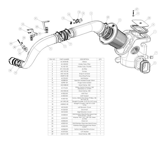
To begin removing the OE airbox, remove the screw fastening the rear of the intake box to the vehicle near the driver side fender.
