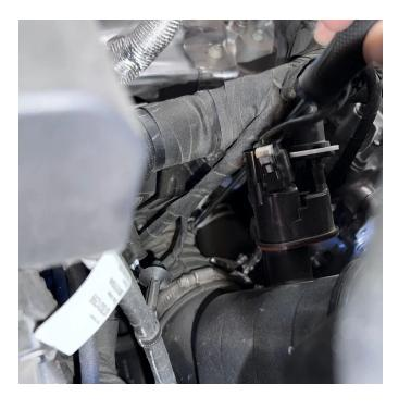
Unfasten the 2 nuts that secure the intake tube to the engine, these will be reused later.
