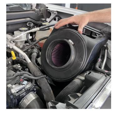
Install the curved intake tube into the vehicle, fitting the coupler over the throttle body.
