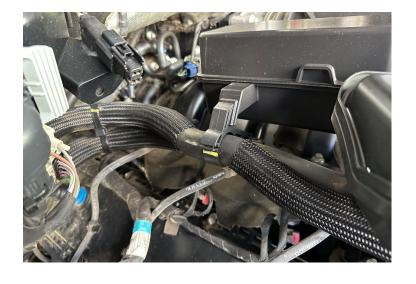
Remove the stock intake tube by disconnecting the tube side from the air box. Then you will pop up the resonators from the grommets
