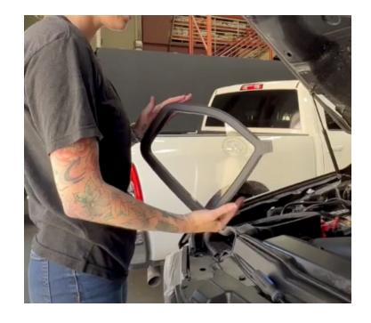
Install the snap-in lid onto the S&B airbox.
