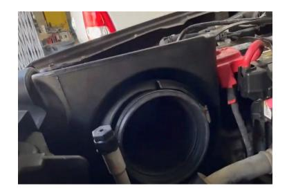
Install the S&B intake tube.
