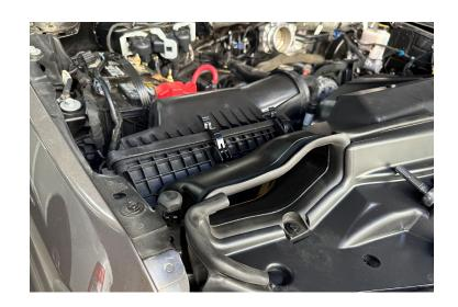
Install the washer and screw onto the bottom of the S&B airbox and tighten down.
