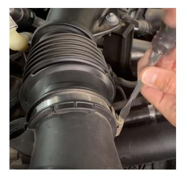
Remove the bolt holding the intake tube down.
