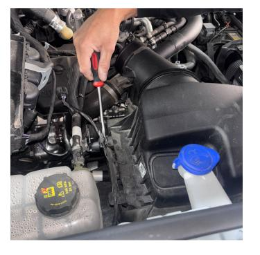
Loosen the hose clamps from the air box end of the turbo intake tube.
