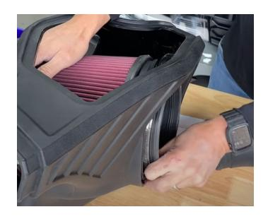
Install the silicone air scoop on the front of the air box.
