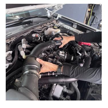
Remove the screw holding the air scoop.
