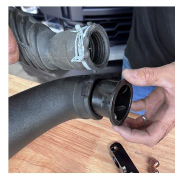
Install the temp sensor grommet into the small y-intake tube.
