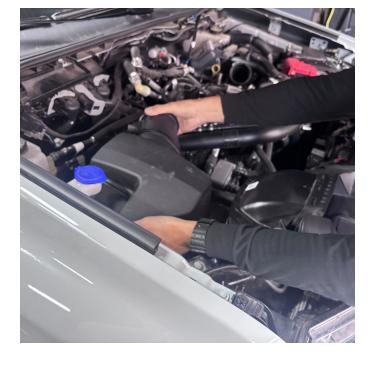
Remove the tube from the Turbo inlet side by using a set of needle nose pliers or vice grips to expand the ring holding the tube.
