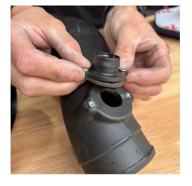
Install the PCV hose connector with corresponding gasket to the long intake tube.
