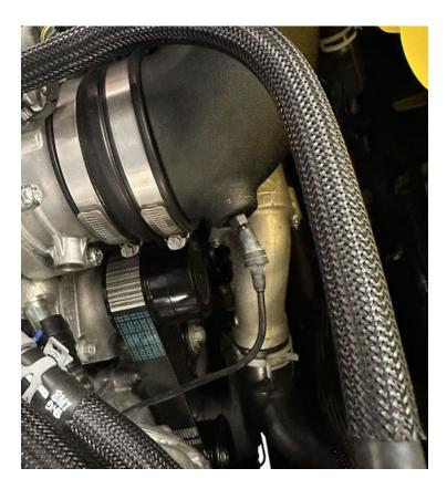
Clip in the quick connect and the IAT sensor. Zip tie the IAT sensor harness to the coolant hose.
