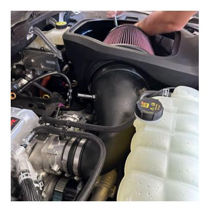
Reinstall the OEM bolt and fender washer. Then fully tighten down.
