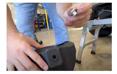
Install the scoop onto the S&B airbox using the provided push rivets.
