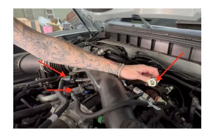
Remove the screw shown in the picture with a 5/16 nut driver or socket.
