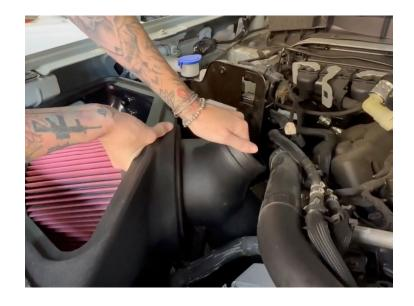
Install the other S&B intake tube into the vehicle. Then tighten down the hose clamps.
