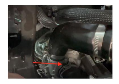
Install the dual quick connect fitting and gasket on the S&B intake tube then tighten down with the provided hardware.
