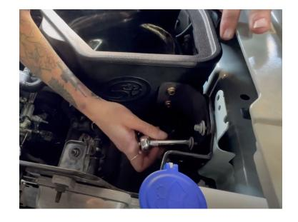
Install the S&B air filter into the airbox.
