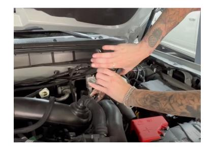
Remove the stock intake tube from the vehicle.
