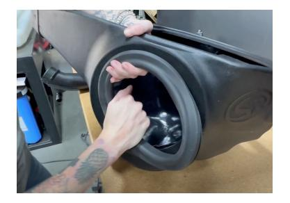
Install the bracket onto the S&B airbox, then tighten down with the provided hardware.
