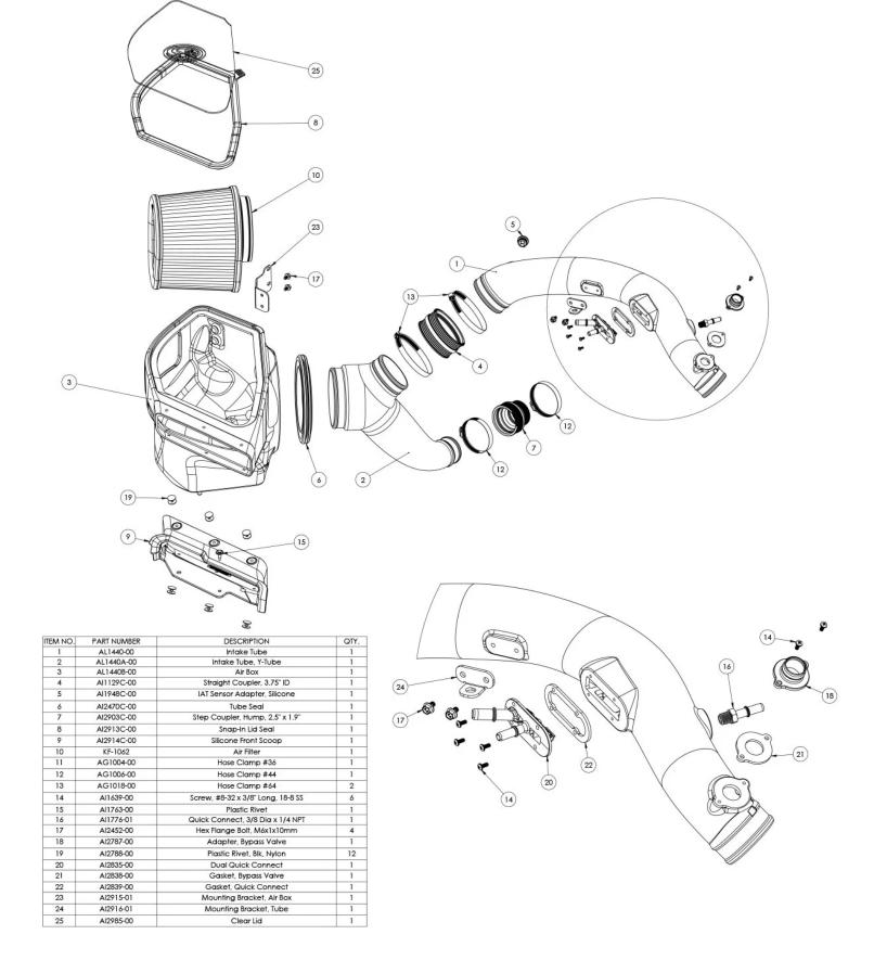
that are attached to the long upper intake tube.
