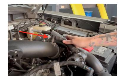
Slide the clamp back over and clamp down to tighten.
