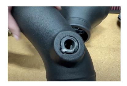
Install the IAT sensor onto the S&B tube, make sure the tab backs up against the ramp as shown in the picture.
