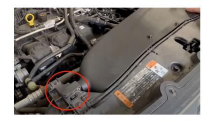
You may now slide the coupler (from the tube that is connecting to the Turbo) over to the main intake tube and connect the two. Make sure the bracket aligns properly.
