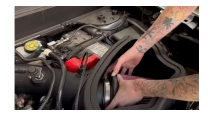
Go back and make sure all Fittings, Clamps, and Harnesses were properly tightened
