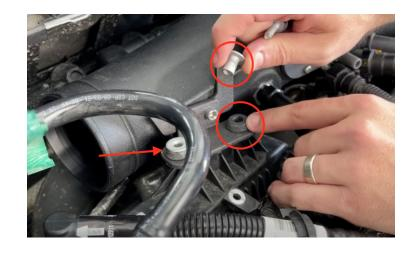
Install brackets on both sides of the S&B scoop
