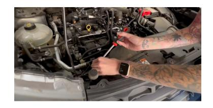
Loosen the Airbox hose clamp, and the IAT sensor.
