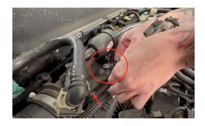
Remove the (2) quickconnect fittings by pulling on the clip (in an outward motion). This will open the clip and allow you to remove the fittings.
