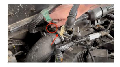
Disconnect the (2) factory Quick-Connect hoses. Pulling the hose out from the base should release and disconnect the hose.
