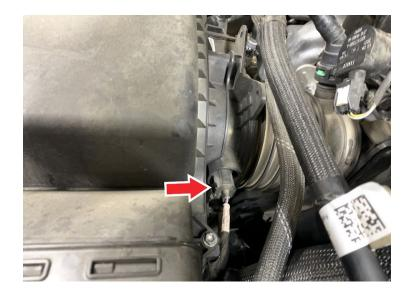
Remove the ribbed push-in retainer clips from the intake box. Use a panel popper to carefully remove the retainer clips.
