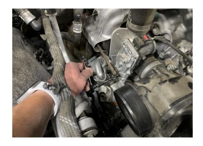
Remove the intake tube from the engine.
