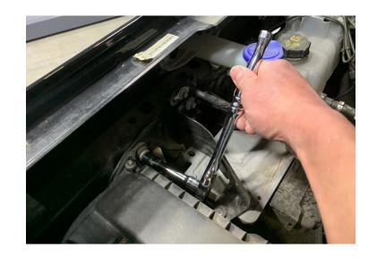
Firmly but carefully rock and lift the intake box free from the lower grommets.Lift and remove the intake box from the vehicle.
