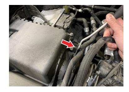
Pull out the green colored locking clip by pushing up in the two small green tabs and then pushing the tabs in the direction of the red arrow in the photo. Then remove the quick connect fitting from the flexible intake coupler that is attached to the intake box.
