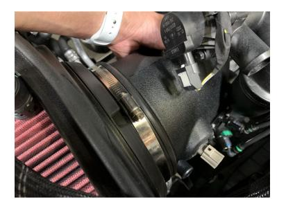
Fully insert the Tube (11) into the Coupler (18) and then move the Hose Clamp (19) into the hose clamp groove on the Coupler and tighten the Hose Clamp.
