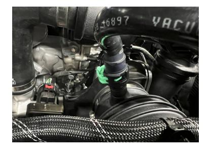
Loosen the hose clamp attached to the flexible coupler.
