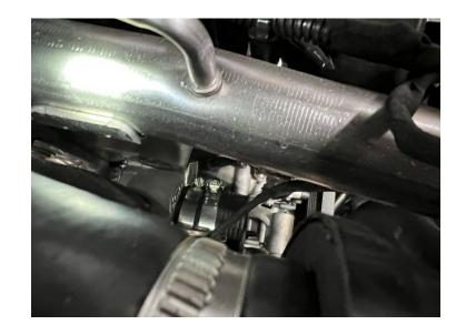
Install tube into the Coupler (18) and then into the Filter (7) flange. Put the Hose Clamp (8) loosely over the Filter flange first. Take your time to carefully snake the Tube into the Coupler first and then work the Tube into the Filter afterwards.
