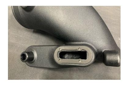
Install Dual Quick Connect (15) over the Gasket (14) making sure the holes of the Dual Quick Connect and Gasket line up with the threaded holes on the Tube. Using Screws (16), fasten and tighten the Dual Quick Connect to the Gasket and Tube.
