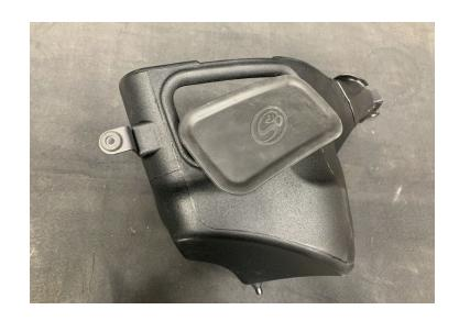
Install the Intake Box (1) into the vehicle. Make sure that the box prongs are aligned with the factory grommets. Push down on the airbox to make sure that the prongs are completely seated.
