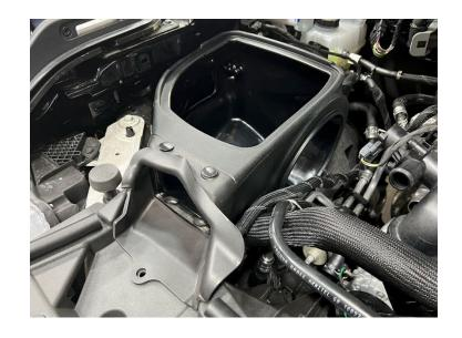
Align the grommet hole in the Box Bracket (2) with the threaded hole in the fender frame and reuse the screw removed in Step 7 to fasten the Box Bracket to the fender frame. Tighten the screw.
