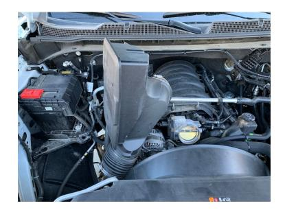
Remove the Crank Case Vent tube from the vehicle. Push down on the gray tab and pull away from the intake.
