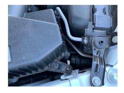
Loosen the hose clamp that secures the intake box to the factory resonator.
