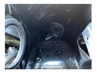
Reinstall the plastic rivet into the factory air scoop.
