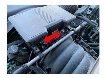
Push down on the gray tab to disconnect the Crank Case Vent line from the resonator.
