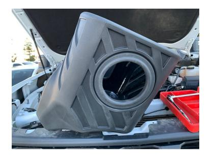
(Optional) Install the box plug into the airbox. (We recommend installing the box plug in warmer climates to ensure your vehicle gets the coldest air possible.
