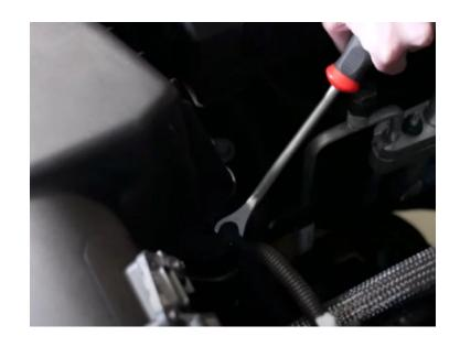
Remove the airbox from the vehicle.
