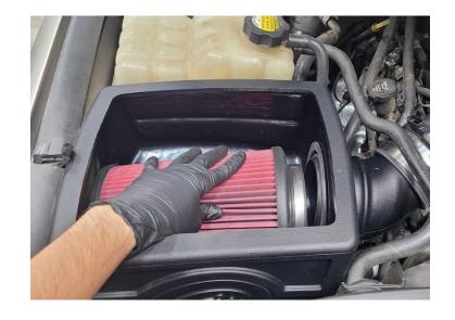
Align the Air Box (E) and Filter to MAF tube (J or Q) with the location arrow.
