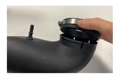
Slide the Straight Coupler (L) over the Intake Tube (M) MAF sensor location along with the #50 Hose Clamp (K), do not fully tighten at this time.
