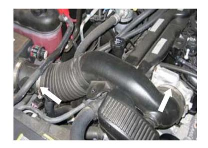
Pull the OE air box towards the engine and up to release it from the vehicle.
