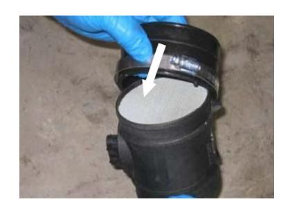
Connect the MAF sensor Assembly (Step 15) to the Filter to MAF Tube (J or Q) and secure using a #50 Hose Clamp (K).
