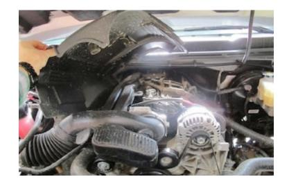
Disconnect the crankcase vent line from the intake tube plenum by gently pulling it out.
