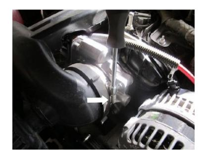
Using a flat blade screwdriver, remove the intake tube from the pushpin located on the coolant tube.
