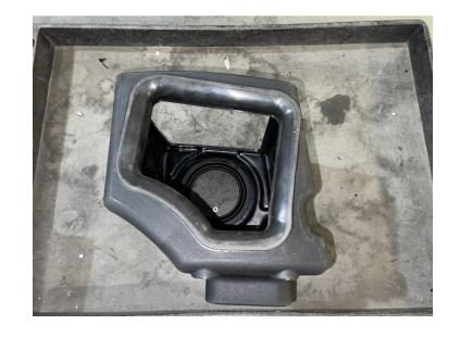
Determine whether or not you would like to install the box plug by reading the Airbox Plug Testing section in the top part of these instructions. If you would like to, install the Box Plug (H) into the Airbox (G)
