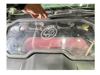
Place the driver's side and passenger's radiator closeout into position over the intake and engine. Place the front cover over those two closeouts. Install the included plastic reusable rivets into the S&B radiator cover hole positions.
