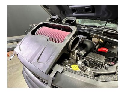
Tighten the air filter onto the S&B intake tube with the hose clamp from Step 24.
