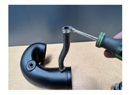
Install the coupler and hose clamps onto the S&B Tube.
