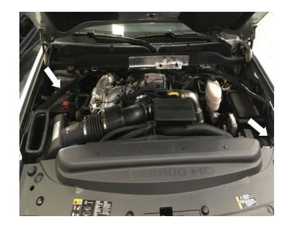
Disengage the red locking clip, press down on the tab, then pull out to disconnect the electrical harness from the MAF sensor.
