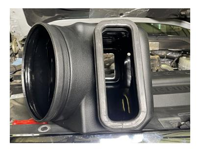
Determine if you want to install the Box Plug (L) onto the Intake Box or leave it open.
