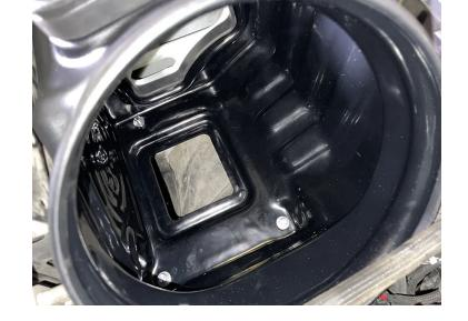
Install the filter (B) into the intake box (A). The lip of the filter should go over the flange on the box and snap onto it.
