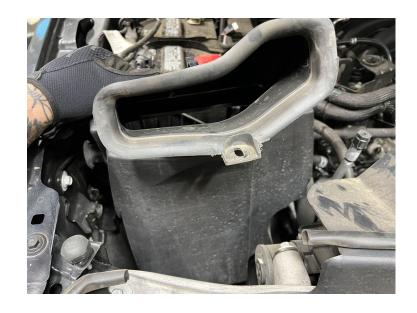
Remove the two screws that hold the saddle bracket and remove the bracket from the vehicle. Set the screws aside, they will be reused Tools Required: 13mm Socket/Wrench Tools Required: 13mm Socket/Wrench.
