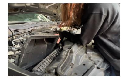
Carefully remove the stock intake filter.
