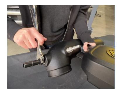
Install the Washer to the bottom of the Air Box using Hex Flange Bolt Tools Required: 10mm Socket/ Wrench or Box/Open Wrench
