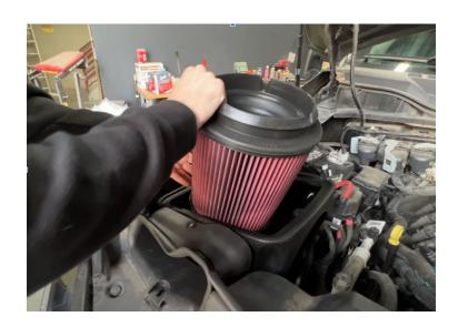
Make sure the filter is snapped into the airbox opening, then pull the filter flange back out. Place the hose clamp on the filter flange but do not tighten it at this time.
