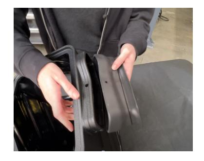
Step 21 Squeeze the Plastic Rivets together so they lock into place through the airbox and Air box inlet.
