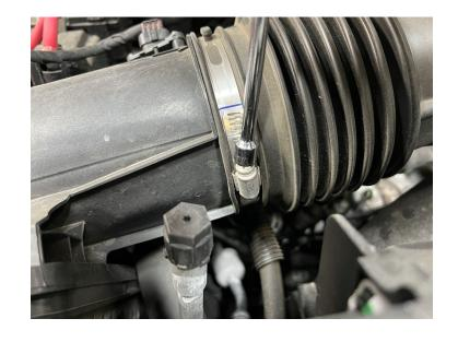
Disconnect the vent lines from the stock intake tube by depressing the latching areas on the quick-connect fittings.
