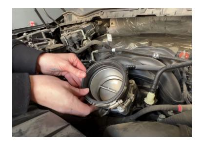
Push the tube into the throttle body and air filter flange.
