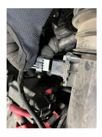
Remove the ribbed push-in clip on the wiring harness from the stock intake lid.
