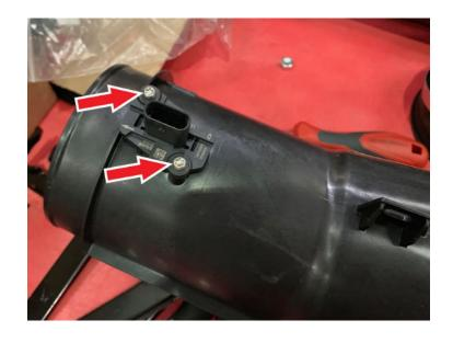
Make sure the stock gasket is on the MAF sensor and place the MAF Mount first and then the MAF Mount Gasket second onto the stock MAF sensor as shown.
