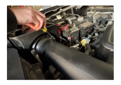
Reconnect both vent lines to the fittings on the S&B intake tube.
