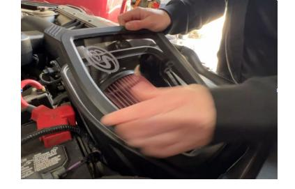
Inspect your installation, and ensure the kit is positioned correctly and all fasteners and hose clamps are secured. Keep all stock parts if you ever need to reinstall the stock intake assembly. Affix the ID label near the Intake kit. If you are an installer, give the owner the QR code for the Installation Instructions so that he/she is aware of the Maintenance and Operation procedures are given at the beginning of the Instructions. The installation is now complete.
