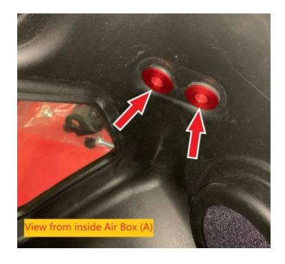
Install Box Seal (M) to the Air Box (A). Make sure that the Air Box (A) is fully seated into the groove of Box Seal (M).
