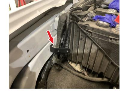
Carefully work the Air Box (A) into the vehicle. The space is tight but carefully move/rotate the box to make space for the grill inlet duct, fender, and coolant reservoir as you lower the Air Box. Once the Air Box is below the fender it will become easy to position the Air Box properly then push down to fully seat the Washer (D) into the stock bottom box grommet shown in Step 12. The AirBox should snap into the grommet.
