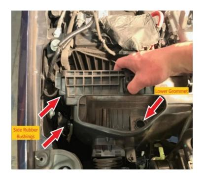
Make sure the bottom box grommet stayed in the vehicle and did not get pulled out with the intake box.
