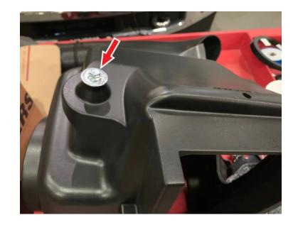
Install Foam Filter (J) and Foam Retainer (K) to the Air Box (A) using M4 Screws (L).
