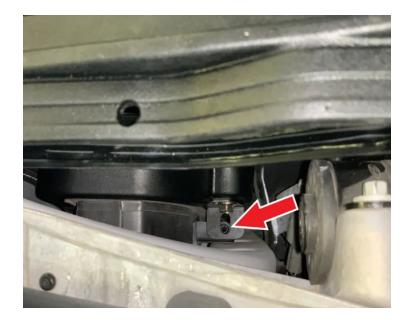
After the holes in both Step 23 and Step 24 are aligned, reuse the OE saddle bracket screw removed in Step 13 to fasten the Air Box (A) to the fender frame. Use the M8 Screws (G) to fasten the Shoulder Bushings (F) to the Air Box Bracket (H). Tighten all fasteners.
