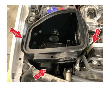
Position the Air Box so that the hole in Air Box (A) is in line and matched with the threaded hole in the fender frame and the holes in the Shoulder Bushings (F) are also in line and matched with the threaded holes in Air Box Bracket (H). Rotate the Air Box Bracket (H) as required.
