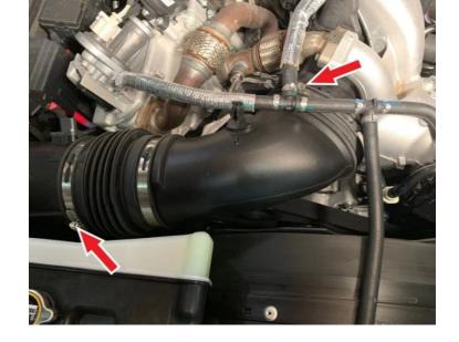
Remove the coolant line from the intake tube clip then remove the intake tube from the vehicle.
