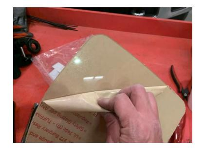
Install the Lid Seal (AD) around the outside edge of the clear Lid (AE).
