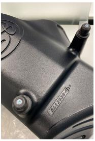
Install the Airbox into the vehicle, sliding the prongs into their holes and lowering the box onto the stud. Reinstall the nut with captive washer onto the stud from the inside of the S&B Airbox.
