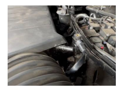
Remove the connector attached to the intake tube by depressing the white button and pulling off. Disconnect the electrical connector next to the PCV connector by sliding out the grey tab and depressing the button
