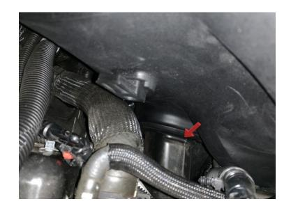
Reattach the unique push clip for the air inlet tube and reinstall the support bracket.
