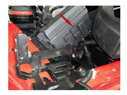
Reinstall the fuse box bracket. Ensure the fuse box is near, but not attached to the bracket.
