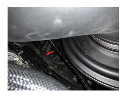
Connect the MAF Harness Extension Cable to the stock MAF Harness and tighten the Push In Cable Tie.
