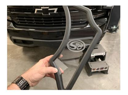
Install the lid and lid seal into the airbox starting from the tight corners and curved edge, working to the straight side.
