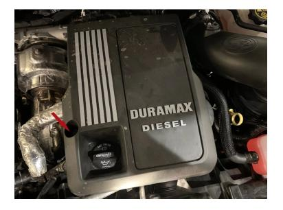
Install the plug (27) into the socket access hole on the airbox.
