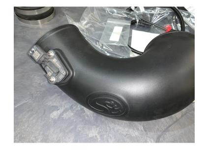
Insert the Short S&B Intake Tube into the Straight Coupler, then insert the tube into the Filter flange. Tighten both hose clamps.
