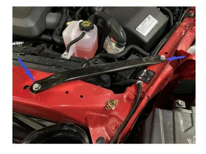
Remove the bolt holding down the front coolant overflow tube.
