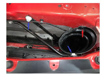
Tighten down the nut with a captive washer to secure the airbox.
