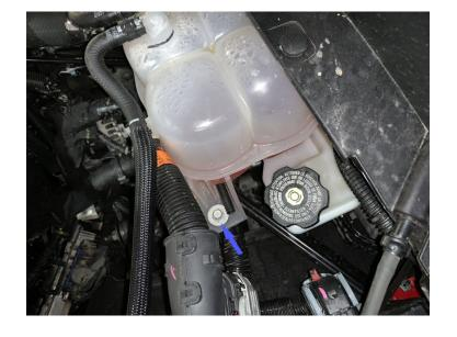
Loosen the hose clamp closest to the turbo inlet on the stock tube. The access to this hose clamp is very limited, caution and patience are required.
