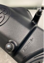
Install the Airbox into the vehicle, sliding the prongs into their holes and lowering the box onto the stud.
