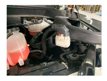
Insert the push clips into the small holes in the S&B Air Box.
