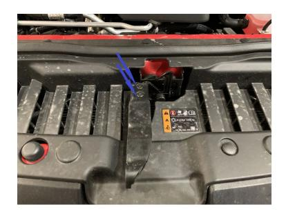
Remove the push clips holding down the large plastic air diverter. Remove the large plastic air diverter and set aside.
