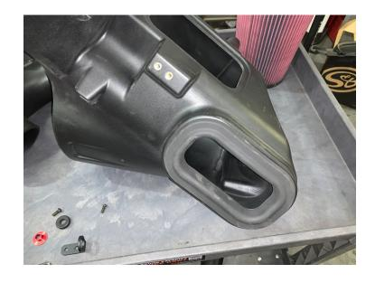
Attach the Harness Bracket (6) onto the airbox with the ¼ x 20 Button Head Cap Screw (17).
