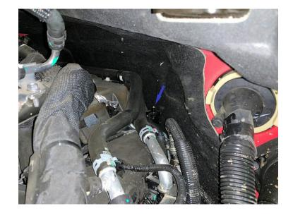
Reinstall rear coolant reservoir and mounting bolt.
