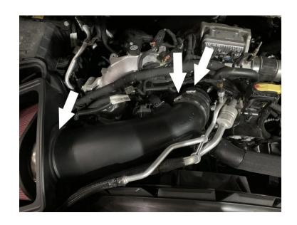
Rotate the filter around the end of the intake tube into the position shown so that it does not contact any walls of the airbox and then tighten the #54 hose clamp (G) located around it's flange.
