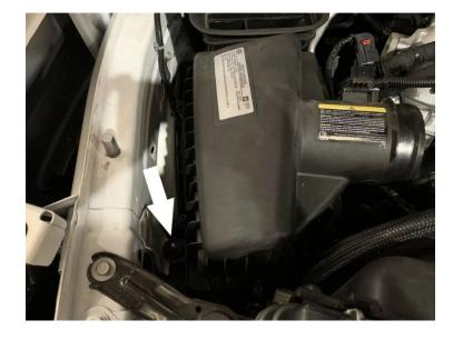
If the grommets are pulled out of the vehicle with the removal of the airbox, pull them off of the airbox prongs and reinsert them into their holes in the engine bay.
