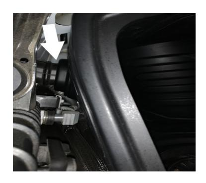
Ensure that the #56 hose clamp (G) is loosely attached around the flange of the air filter and place the air filter (D) into the airbox through the top opening. Make sure that the end of the filter opposite of the flange is pointed toward the rear of the vehicle.
