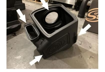
Install the S&B airbox into the vehicle, verifying that the threaded stem shown travels through the shoulder washer installed on the last step. Replace the nut removed in step 5 to secure the airbox to the vehicle.
