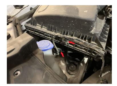
Remove the hose clamp connecting the tube to the resonator .
