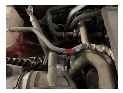
Remove the bolts holding down the air intake scoop.
