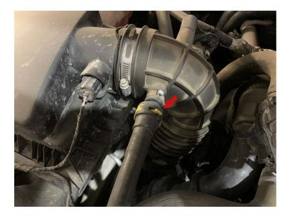
Depress the locking bottom and disconnect the electrical connector.
