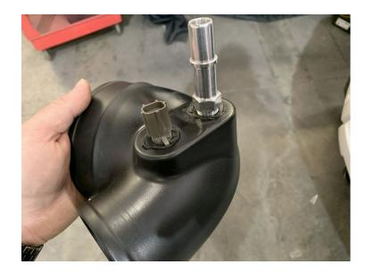
Install the rubber mounting prong grommet(#9) onto the bottom of the airbox
