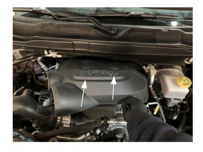
Disconnect the crankcase vent tube by pulling the hose firmly away from the factory air tube.
