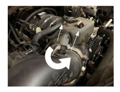
Using a 5/16" driver or socket, loosen the hose clamp on the factory tube connected at the throttle body.
