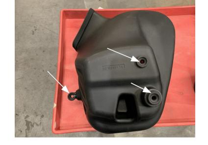
Remove the top portion of the factory scoop by prying the tabs to the sides of the scoop from the factory intake assembly using a flathead screwdriver.
