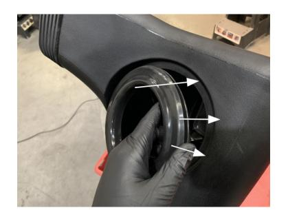
Push the S&B Tube (M) through the Silicone tube seal (L)
