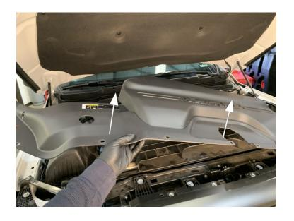
Remove the 2 bolts attaching the factory air scoop to the vehicle using a 10mm socket and driver. Collect these bolts and set them to the side, to be reinstalled later.
