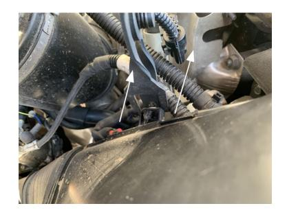
Firmly Lift up and remove the entire factory intake assembly from the grommets of the vehicle. Set the assembly to the side
