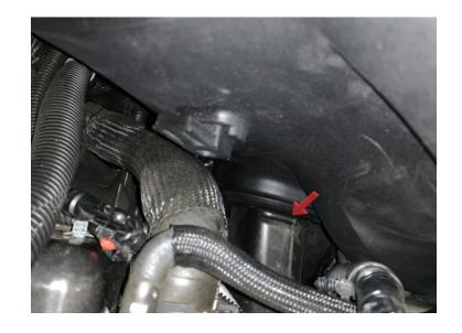
Reattach the unique push clip for the air inlet tube and reinstall the support bracket.
