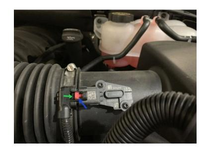
Disconnect the crankcase vent tube at both ends by pressing down on the grey quick disconnect buttons.
