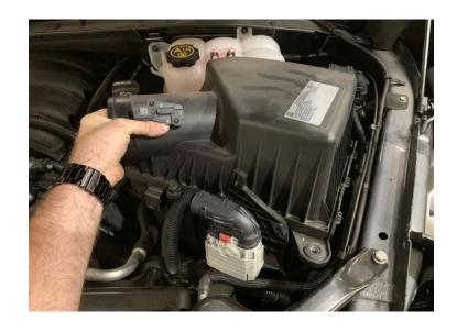
Find the S&B Air Intake Box (1) and the Silicone Inlet Seal (3). Install the Inlet Seal onto the Airbox.
