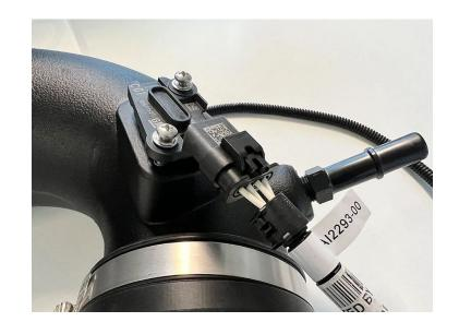
Snap-in a Push-In Cable Tie (26) into the insert on the back of the intake tube.
