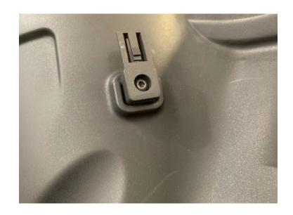
Install the Panel Grommet (16) into the Airbox. Install the Machined Aluminum Shoulder Washer (15) into the Panel Grommet.
