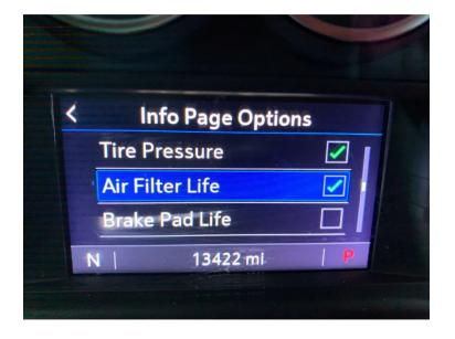
Navigate to the Info section of the Driver Information Center, and scroll down to the Air Filter Life section. Press the wheel in to select the Menu for the Air Filter Life, and select Disable.
