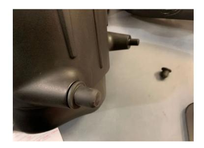
Install the Airbox into the vehicle, sliding the prongs into their holes and lowering the box onto the stud. Reinstall the nut with captive washer onto the stud from the inside of the S&B Airbox.
