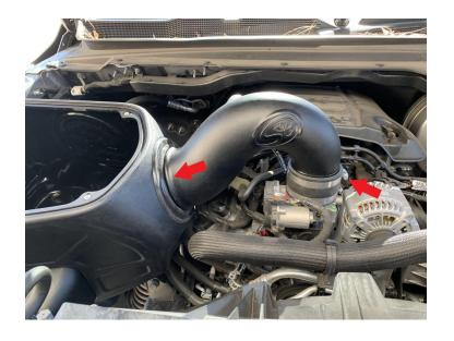
Install the Air Filter (H) onto the Intake Tube (B) and tighten the #88 Hose Clamp (O). Do not overtighten.
