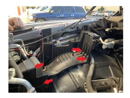
Remove the four bolts securing the intake box tray. Set two bolts aside, they will be used in Step 21.
