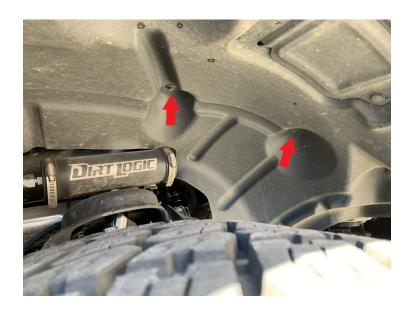
Lift the intake box to unseat the grommets from the intake box tray then remove from the intake box from the vehicle.
