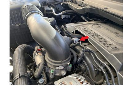
Loosen the hose clamp at the throttle body then pull the intake tube away from the throttle body.
