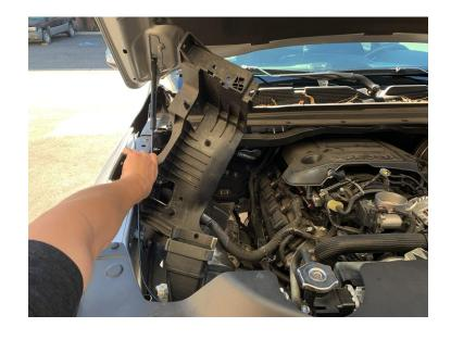
Install the Tube Seal (E) onto the Intake Box (A).
