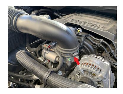
Loosen the hose clamp at the intake box then completely remove the intake tube from the vehicle.
