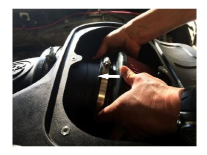
Tighten the Hose Clamp #88 (J) at the Air Filter (D).
