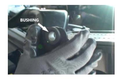
Install the grommet into airbox (A) first and then install the metal bushing from the inside.
