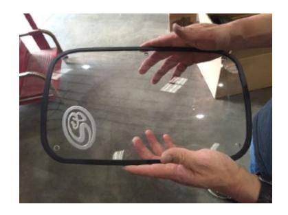
Install the Clear Lid (E) on top of the airbox (A) and secure the lid using the six provided Truss Head Phillips Screw (M) and Sealing Washer (L). Do not over tighten.
