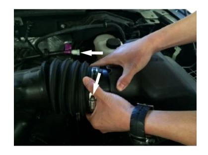
Unlatch the two latches on the stock airbox.
