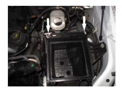
Remove the plastic rivets on the stock air scoop using a flat head screwdriver
