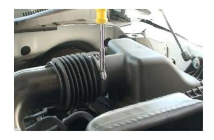
Loosen the hose clamp at the tube leading to the turbo inlet on the passenger side.
