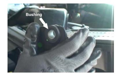
Install the grommet into airbox (A) first and then install the metal bushing from the inside.
