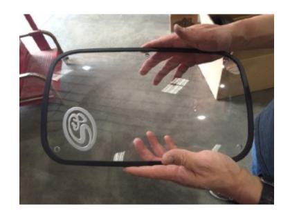
Place the lid on top of the airbox (A) and secure the lid using the six provided 10-24 Screw (N) and Sealing Washer (M). Do not over tighten.
