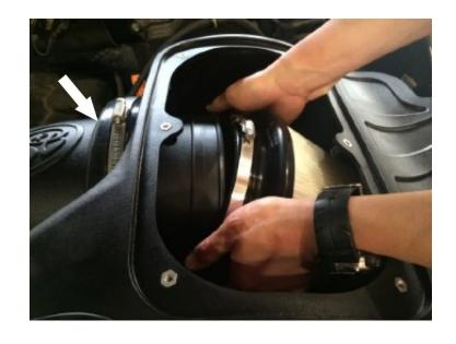
Tighten the Hose Clamp #88 (K) at the Air Filter (D).
