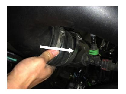
Slide the Hump Coupler (P) over the passenger side turbo inlet tube.
