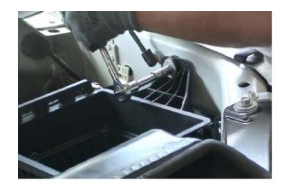
Remove the plastic rivets on the stock air inlet using a flat head screwdriver.
