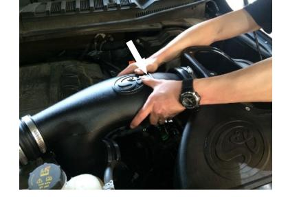
Once the bead is up to the Cuff (C). Slide the Air Filter (D) onto the Intake Tube (B).
