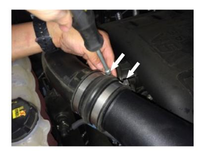
Tighten both #72 Hose Clamps (T) on the driver side.
