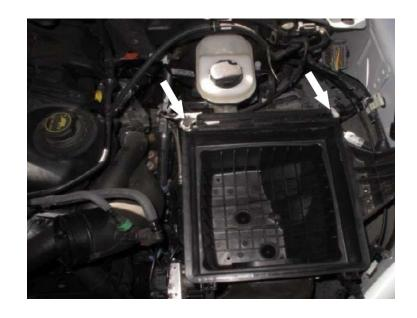
Lift and remove the stock airbox.
