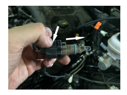
Lift up and remove the stock air tube.
