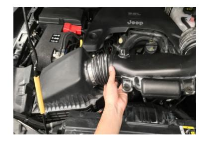
Check to make sure the two grommets are still in place.
