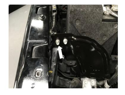
Install the IAT Sensor Grommet (J) into the Intake Tube (B).
