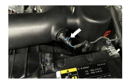
Connect the CCV hose into the Quick Connect Fitting (I). You should hear a snapping sound when the CCV hose is fully secured
