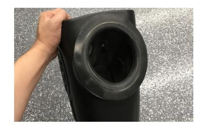
Install the Tube Seal (D) onto the Intake Box (A).
