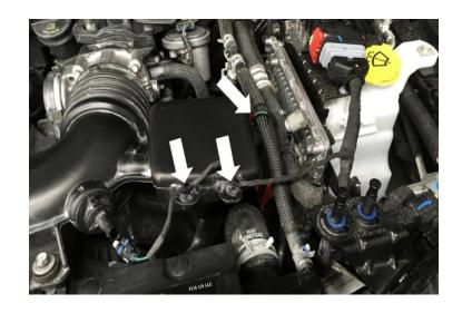
Remove the two bolts securing the stock intake tube to the fan shroud.
