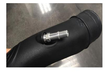
Install the Coupler (E) with the two #56 Hose Clamps (N) onto the Intake Tube (B) then tighten the hose clamp closest to the intake tube. Do not overtighten. Leave the hose clamp for the throttle body loose.
