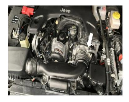
Remove the bolt securing the stock intake box to the fender.
