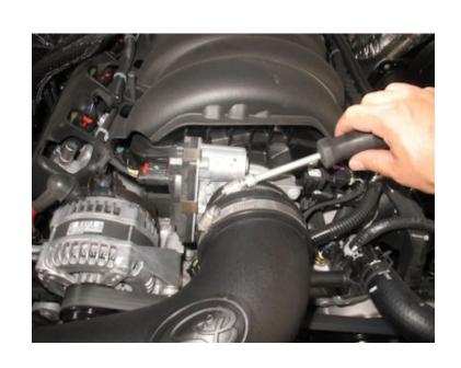
Connect the MAF harness to the MAF sensor. Make sure the red locking latch is secure.
