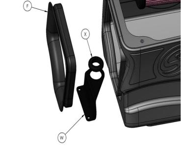
Note: If you have vehicles equipped with HID headlights proceed to Step 19, otherwise continue with Step 18. Install the Airbox (A) and remember to properly align the fender seal to the side fender opening. Secure the airbox and Filter Support Bracket (W) with the M6 Bolts (L) and Washers (K). Make sure all fasteners are tightened. Go to Step 22.
