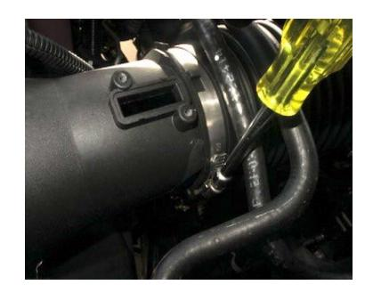
Once the hose clamp is loose, pull tube to the right to remove from factory airbox cover.
