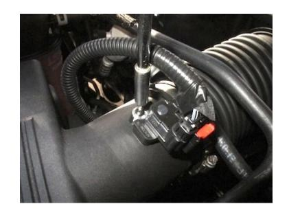
Once the sensor is removed, disconnect the sensor from the harness by pulling the Red tab out and pressing down on the release button while pulling out. Place the sensor in a safe location for later install.
