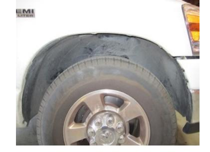
From inside the engine compartment, carefully pull the wiring harness clip out of the wheel liner. Then set the wheel liner aside.
