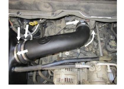
Reconnect the temperature sensor wiring harness into the sensor
