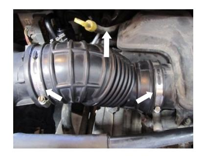
Loosen the two screws on the resonator assembly using a 10mm socket. Disconnect the temperature sensor wiring harness from the sensor.
