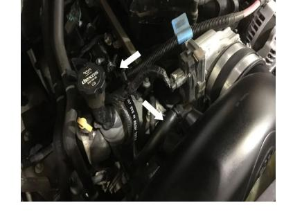
Reconnect the MAF harness back into the MAF sensor and engage the red locking clip.
