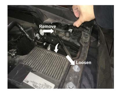
Loosen the hose clamps at the throttle body and airbox. Do not remove the intake tube yet.
