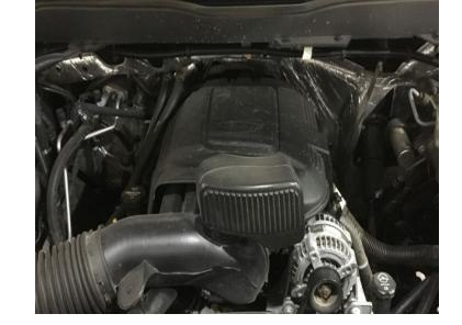
Disengage the red locking clip and disconnect the MAF sensor harness from the MAF sensor. Pop-out the harness clip attached to the stock airbox.
