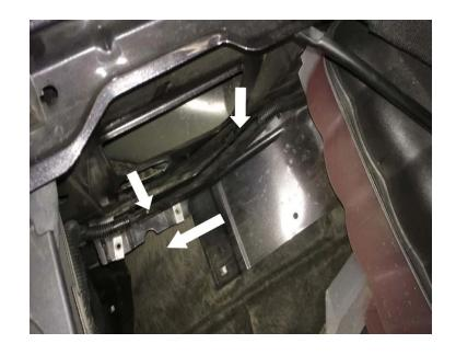
Install the Tube Seal (H) onto the Airbox (A).
