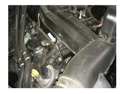
Remove and set aside the two plastic push pins on the passenger side of the radiator shroud to access the front bolt securing the cross member. The plastic push pins will be reused in Step 27.
