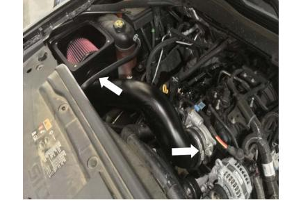
Install the Air Filter (B) onto the Intake Tube (I) and tighten Hose Clamp #88 (G). Position the air filter in the same position as shown below.
