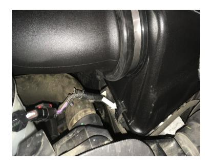
Install the Throttle Body Intake Tube (L) into the couplers on the throttle body and Air Filter Intake Tube (I). Make any final adjustments and tighten all #60 Hose Clamps (J).
