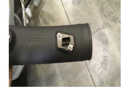
Install the Coupler (K) with the #60 Hose Clamps (J) onto the throttle body. Tighten the hose clamp on the throttle body side only. Leave the other one loose.
