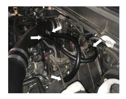
Connect the other end of the MAF Extension Harness (U) into the MAF sensor.
