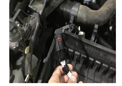
Install the intake assembly into the factory intake box. Make sure that the tabs on the Intake Box Cover (C) are lined up with the slots on the factory intake box. Once the tabs are in the slots lower the whole intake assembly. Proper installation into the slots will reduce any vibrations.
