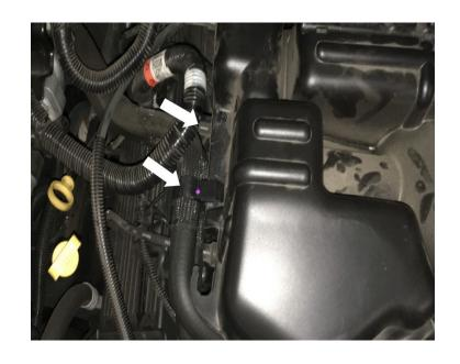
Remove CCV hose #1 from both the stock resonator intake tube and the hose barb near the firewall.
