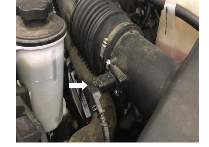
Pop-out the two harness clips on the passenger side from the stock resonator intake tube.
