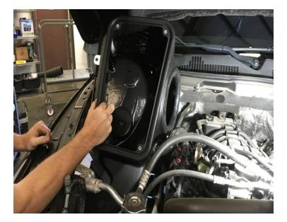
Install the M8 Screw (Q) and Washer (P) through the Mounting Bracket (D) to secure the Air Box (A). Do not fully tighten yet.
