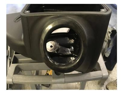
Install the Grommet (H) onto the Air Box (A).
