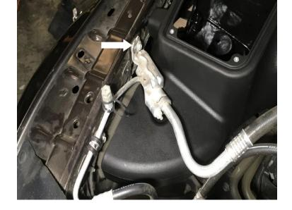
Reconnect the sensor into the wheel liner from Step 9 and secure the wheel liner with the airbox with the 1/4-20 Screws (O), Washers (N), and Locknuts (M). Leave the Screws loose so adjustments can be made while reinstalling the wheel liner. Reinstall the wheel liner and the screws. Use the Panel Retainer Pins (W) to replace any pins broken during the removal process. You will need two 11mm Socket or Wrench to tighten both the screw and locknut.
