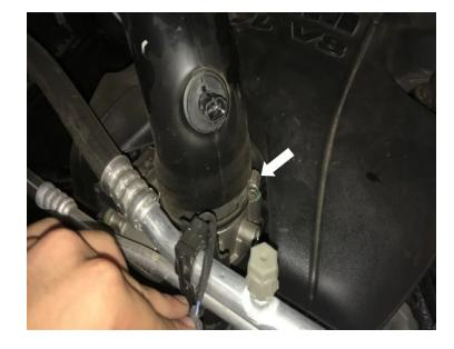
Loosen the clamp connecting the intake tube to the intake box then remove the intake tube from the vehicle.
