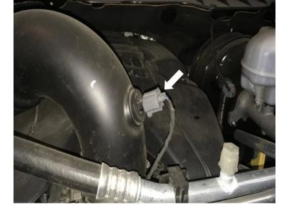
Disconnect the crank case vent tube from the air box.
