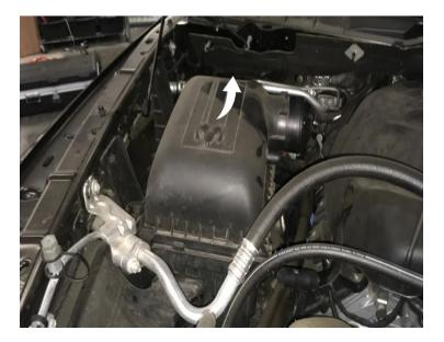
Lift up to remove the engine cover from the vehicle. If necessary remove the oil cap if it gets in the way.
