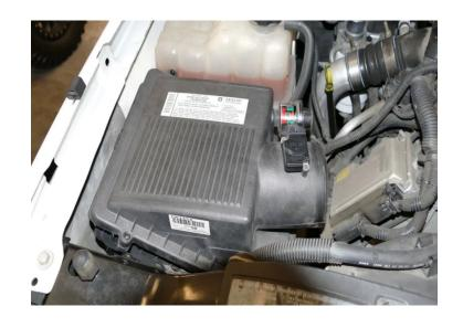
Remove the five screws securing the factory airbox tray with a 10mm Socket or Wrench.
