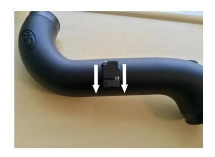
Slide the Coupler (T) and two #72 Hose Clamps (J) onto the Intake Tube (H). Tighten the hose clamp closest to the tube. Leave the other end loose.
