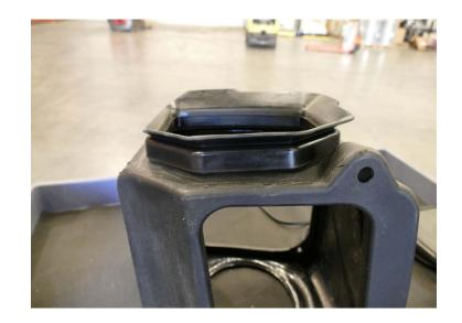
Carefully remove the MAF sensor from the stock intake tube with a T20 Safety Torx. Use the provided Foam Gasket (R), MAF Plate (Q), and 8-32 Screws (K) to install the MAF sensor onto the Intake Tube (H) with a Screwdriver. The MAF sensor should be installed in the same orientation as shown below.
