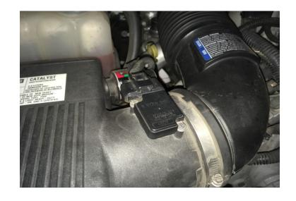
Remove the stock intake tube from the vehicle.
