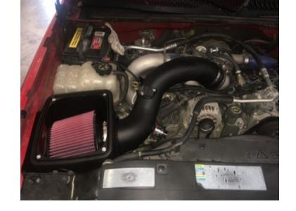
Slide the Air Filter (D) onto the Air Tube (H) and tighten the #80 Hose Clamp (I). Install the Lid Seal (C) into the Air Box (A) grooves.
