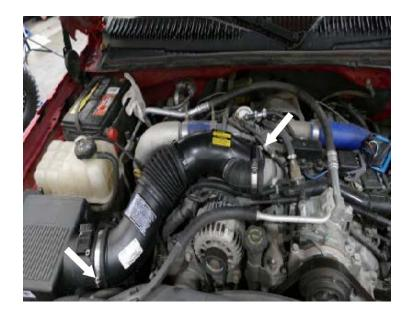
Remove the stock intake box by lifting up to unseat the two prongs from the airbox tray underneath.
