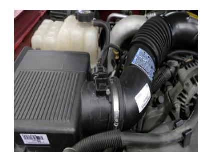
Remove the stock resonator from the vehicle by loosening the bolt and the hose clamp.
