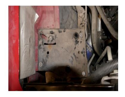
Remove the stock foil from the inner fender. This will allow for additional airflow with our kit.
