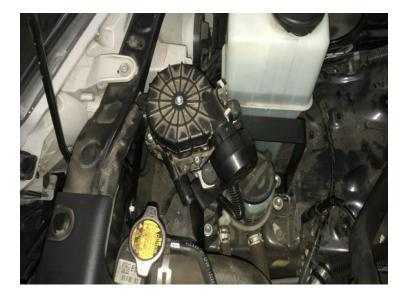
Rotate the smog pump hose at the engine inlet until there are no kinks and reconnect the hose into the smog pump.
