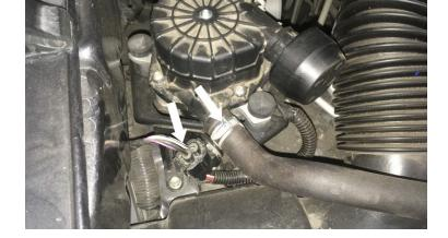
Remove the three bolts securing the smog pump bracket then remove the smog pump and bracket assembly from the vehicle.
