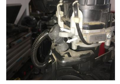
Apply even pressure and carefully slide the grommets out of the bracket. Be careful not to damage the grommets because they will be reused and installed onto the three Smog Pump Brackets (S, T, and U).
