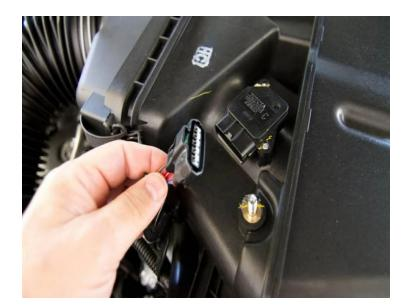
Disconnect the breather and vacuum hoses. Remove the two mounting screws on the intake box. Loosen the hose clamp on the throttle body. Pop-out the wire harness clip.
