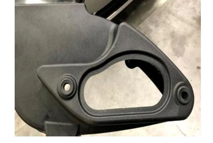
Insert the Airbox Mounting Spacer (16) and Silicone Hose (17) into the corner Grommet (15)
