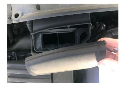
Remove the secondary piece of the inlet scoop
