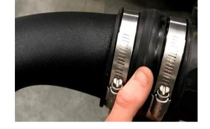
Install the Coupler (1) on the throttle body using the provided Hose Clamp (2)
