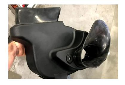
Install the Airbox (8) on the pegs in the engine bay. Make sure to adjust the Base Scoop (18) as needed and adjust the Inlet Seal (14) so that it surrounds the inlet area. You will need to position the coolant hose around the front of the air box as shown below in the picture to the right.
