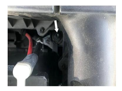
Lift up and remove the stock intake system
