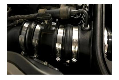
Install the Lid Seal (20) on the Airbox (8)
