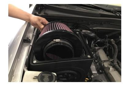
Insert the Intake Tube (E) through the Tube Seal (D) into the Intake Box (A) then slide the Air Filter (C) onto the intake tube. Tighten the #80 Hose Clamp (H).
