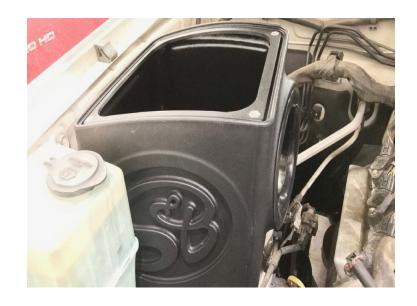
Reinstall the stock screws removed from Step 5 to secure the Intake Box (A). Install an M6 Locknut (R) on the bolt with the hole that is not threaded. Make sure that the bolt goes through the hole through the wheel well cover before installing the locknut from underneath the wheel well.
