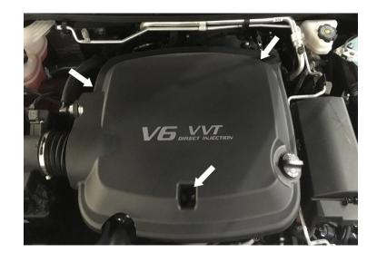
Loosen the hose clamp at the throttle body. The location of the throttle body is closest to the driver's side.
