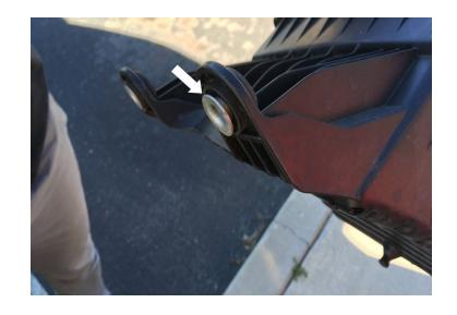
Install the Air Box Grommets (M) into the Airbox (A).
