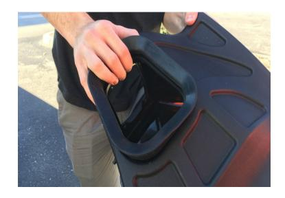
Install the Tube Seal (B) onto the Airbox (A).
