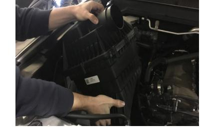
Carefully remove the MAF sensor from the stock intake box lid. Use the supplied 8-32 Screws (C), MAF Pad (D), MAF Gasket (E) to install the sensor onto the Intake Tube (Filter) (L). Do not over tighten.
