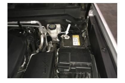
Disengage the red locking clip and disconnect the MAF sensor harness from the MAF sensor.
