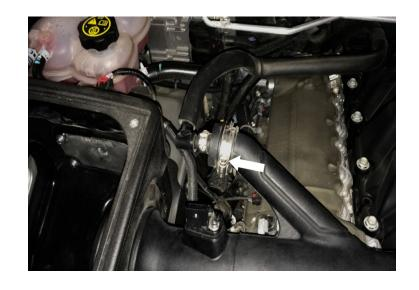
Place the Air Filter (S) into the Airbox (A). Rotate the air filter into position as shown below and tighten the #80 Hose Clamp (X).
