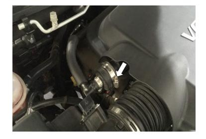
Loosen the hose clamp and disconnect the intake tube from the stock airbox.
