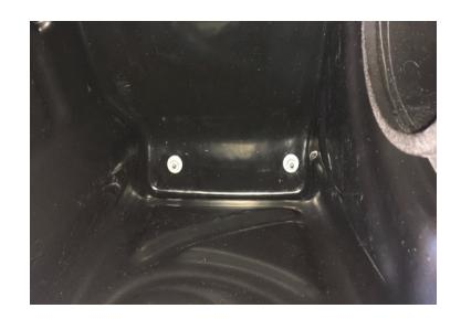
Skip to Step 30 if you installed the Box Plug (P) in Step 23. If you installed the Auxiliary Scoop (O), install the 1/4-20 Screws (L), Lock Washers (M), and Washers (N) from inside the Airbox (A).
