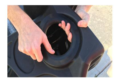
Determine if you want to install the Box Plug (P) "Step 23" or Auxiliary Scoop (O) "Step 24" onto the Airbox (A). See the "Air Box Plug" note to decide if this is the desired setup. To install the box plug, install the 1/4-20 Screws (L), Lock Washers (M), and Washers (N) from inside the airbox then proceed to Step 25.
