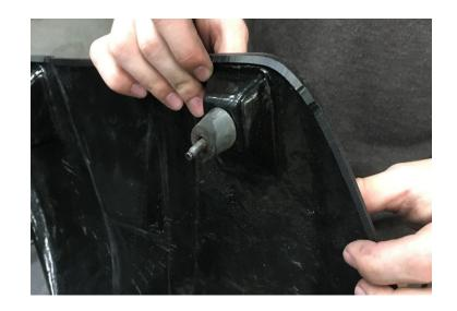
Install the grommet removed in Step 39 onto the mounting location at the side of the S&B Engine Cover (T), then press the metal bushing into the grommet.
