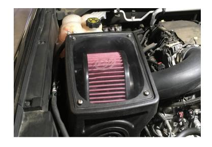
Reconnect the MAF sensor harness into the MAF sensor and engage the red locking clip.
