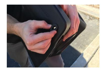
Install the metal bushings removed in Step 18 into the Airbox Grommets (K).
