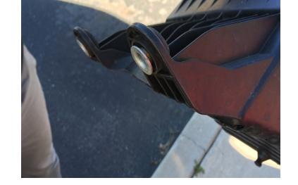
Install the Air Box Grommets (K) into the Airbox (A).
