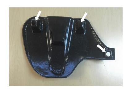
To remove the side mounting hardware on the side, remove the metal bushing first and then the rubber grommet. Set these aside, they will be installed into the S&B Engine Cover (T) in Step 41.
