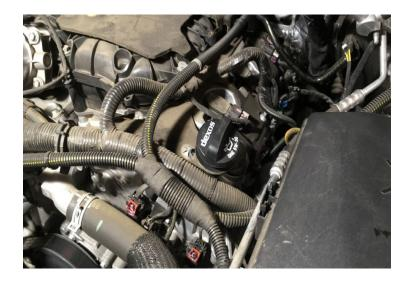
Disconnect the wire harness clip on the stock intake box lid.
