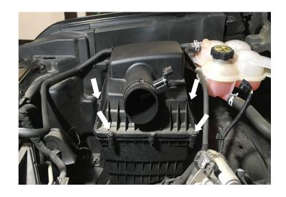
Remove the air filter from the stock intake box.
