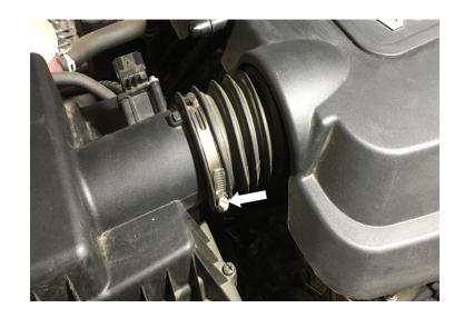
Loosen the hose clamp connected to the throttle body. The throttle body is located underneath the engine cover.
